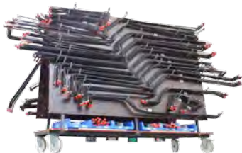
Kanban transport for prefab piping
