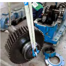
Repair and refurbishment of gearboxes
