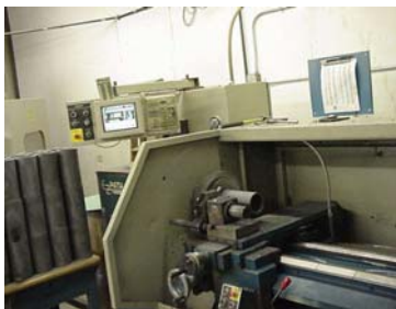
CNC Turning Center - →15" x 30" cap.
