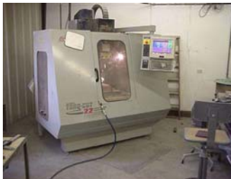
CNC Machining Center - 32 x 16 x 20" cap.
